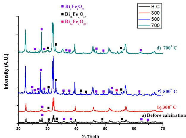
**Fig. 1.** XRD patterns of BiFeO<sub>3</sub>: (a) Before calcination (b) Calcinated at 300°C (c) 500°C and (d) 700°C.
