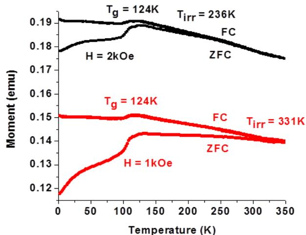
Fig. 5. Temperature dependence of magnetization at H=1kOe and 2kOe of  $\text{BiFeO}_3$  Sample.
