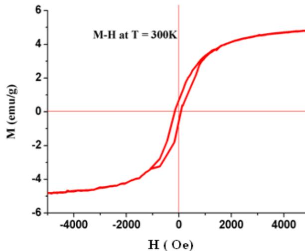
Fig. 4. M-H hysteresis curve for BFO at T=300K.
