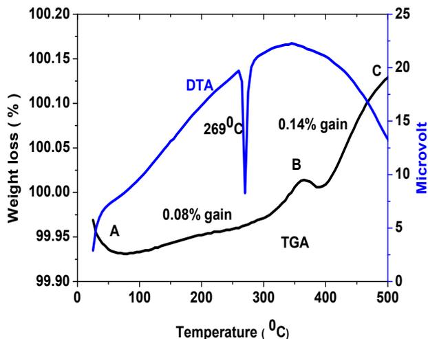
Fig. 3. TGA-DTA spectra of BFO.
