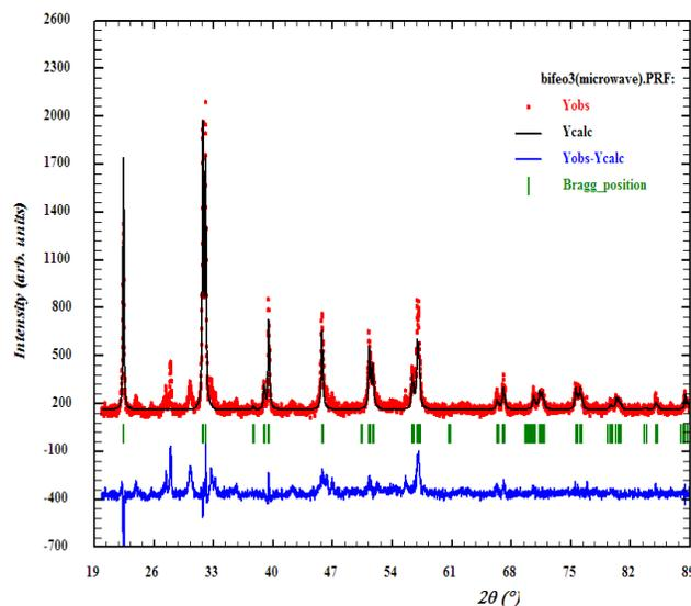
**Fig. 2.** Rietveld refinement of XRD patterns of BFO sample.
