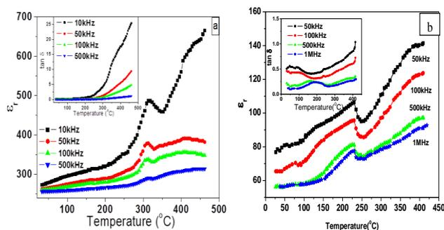
Fig. 2. Temperature dependence of relative dielectric constant ( $\epsilon_r$ ) and loss tangent ( $\tan\delta$ ) at for BSGTV (a) and BSSTV (b) compounds.
