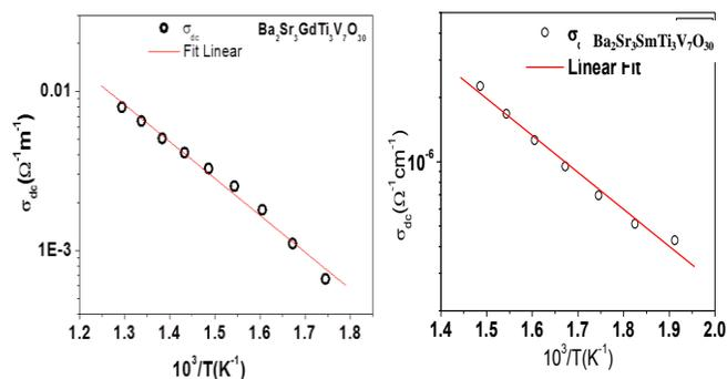
Fig. 3. Arrhenius plots of the electrical conductivity (dc) of BSGTV and BSSTV compounds.
