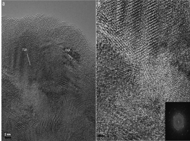
**Fig. 6.** Nanocrystalline structure and electron diffraction pattern of the powder alloy Fe-18Cr-8Ni-12Mn-0,04N after the MA in the nitrogen atmosphere for 3.5 hours.
