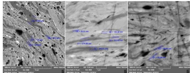
**Fig. 8.** Evolution of the layered structure of the powder particles Fe-18Cr-8Ni-12Mn during MA with the duration of 15 min (a); 30 min (b) and 45 min (c).
