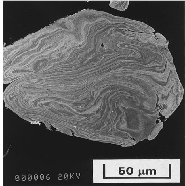
**Fig. 7.** Layered structure of the powder particles in Ag - Cu system, obtained via MA [6].
