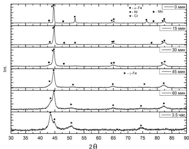
Fig. 1. XRD patterns of the powder Fe-18Cr-8Ni-12Mn-xN at the different mechanical alloying duration.
