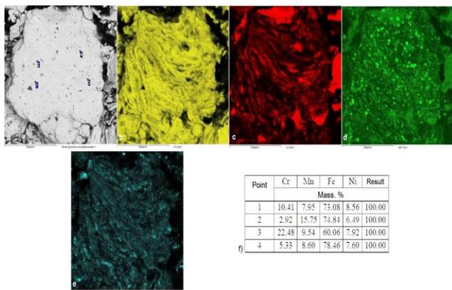
**Fig. 3.** Distribution of components in the particles Fe-18Cr-8Ni-12Mn, after 15 minutes MA synthesis: a - the structure of the investigated area; b - Fe; c - Cr; d - Mn; e - Ni; f - spot chemical analysis results.
