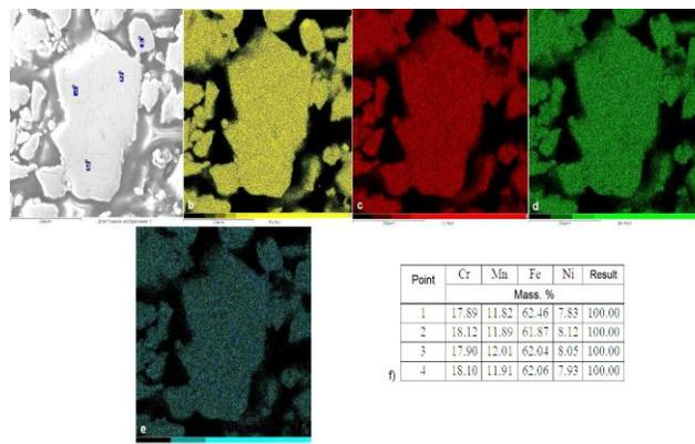
**Fig. 4.** Distribution of components in the particles Fe-18Cr-8Ni-12Mn, after MA synthesis for 3,5 hour: a - the structure of the investigated area; b - Fe; c - Cr; d - Mn; e - Ni; f - spot chemical analysis results
