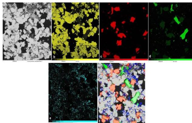
Fig. 2. Distribution of components in the initial powder Fe-18Cr-8Ni-12Mn: a - the structure of the investigated area; b - Fe; c - Cr; d - Mn; e - Ni; f - total distribution of elements.
