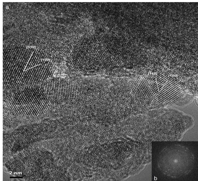
**Fig. 5.** Nanocrystalline structure of the high nitrogen alloy powder with Fe-18Cr-8Ni-12Mn-0,9N, after MA for 3.5 hours in the atmosphere of ammonia (a) and electron diffraction pattern (b).
