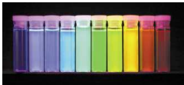
Fig. 4. Ten distinguishable emission colors of ZnS capped CdSe QDs excited with a near-UV lamp. From left to right (blue to red), the emission maxima are located at 443, 473, 481, 500, 518, 543, 565, 587, 610, and 655 nm [20].
