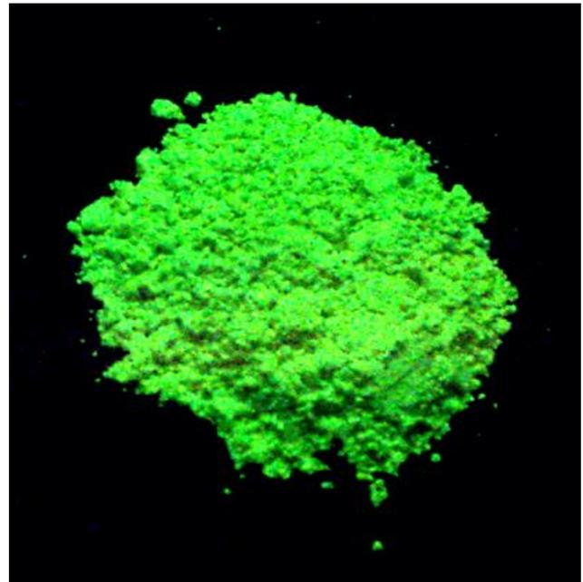
Fig. 6. Green luminescent  $\text{Sr}_2(\text{BO}_3)\text{Cl}:\text{Tb}^{3+}$  powder phosphor under an UV source.
