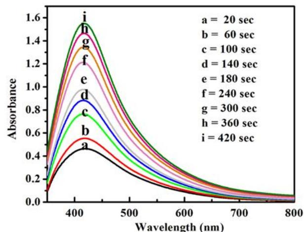
Fig. 1. UV–Vis. spectra of AgNPs showing the SPR peak at 430 nm.
