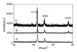
**Fig. 3.** XRD of products prepared at various reaction temperatures of (A) 125°C, (B) 150°C and (C) 180°C.
