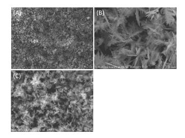
**Fig. 2.** SEM images of products prepared at various reaction temperatures of (A) 125°C, (B) 150°C and (C) 180°C.
