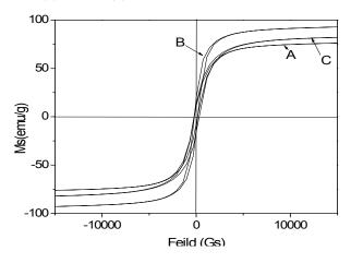
**Fig. 4.** VSM of products prepared at various reaction temperatures (A) 125°C, (B) 150°C and (C) 180°C.
