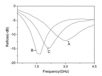
**Fig. 5.** The reflection loss of Fe-Ni alloy prepared at various reaction temperatures (A) 125°C, (B) 150°C and (C) 180°C.
