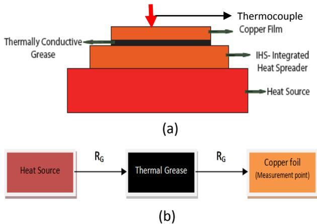
**Fig. 1.** (a) Replica of the experimental setup and (b) Resistance network.
