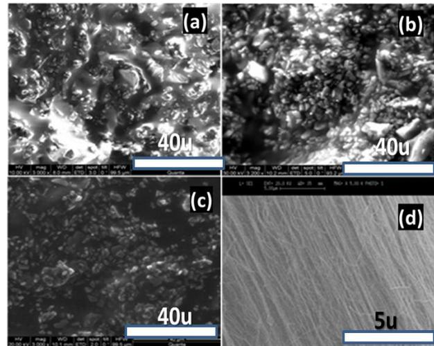
**Fig. 3.** SEM images of grease with (a) 1%, (b) 2%, (c) 4% and (d) aligned MWCNT bundle.
