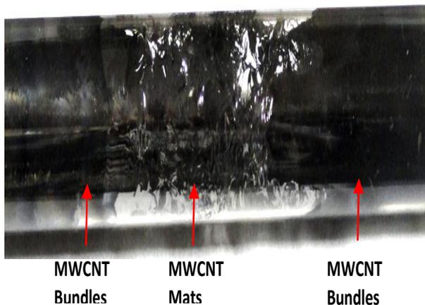
**Fig. 2.** Quartz tube with MWCNT bundles and mats.
