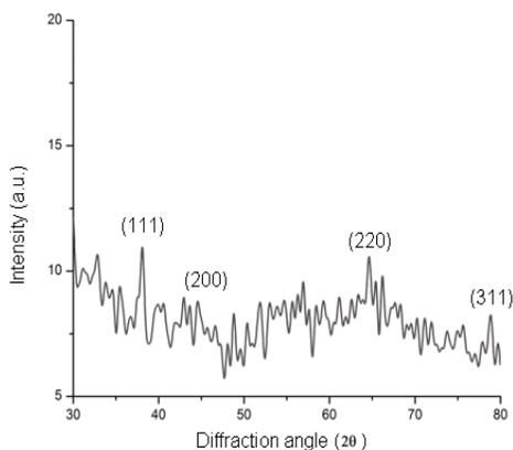
**Fig. 2.** XRD pattern of AuNPs obtained from sample S4
