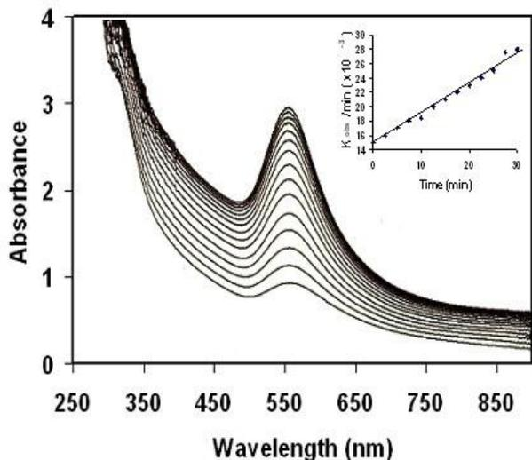
Fig. 6. UV-Visible spectra of AuNPs formation with HAuCl<sub>4</sub> (5.16mM) tea extract (1.5 mL) reduction at 3 minutes time interval
