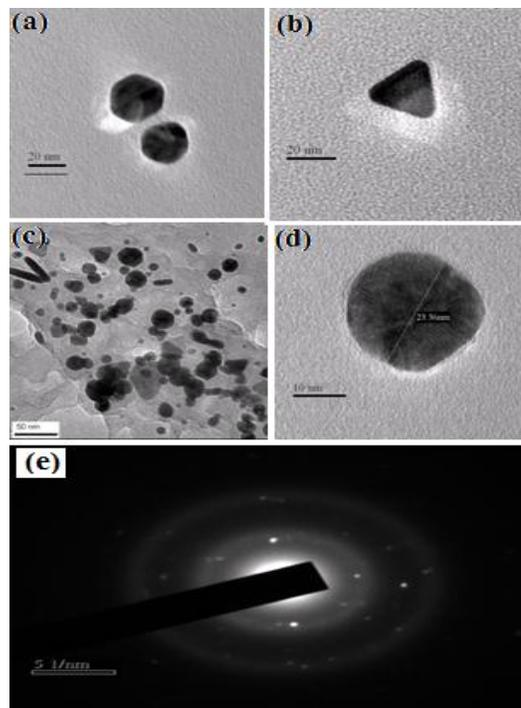
**Fig 3.** (a-d) HR-TEM images of AuNPs sample S4 under different magnification, (a) 20 nm (spherical and hexagonal shape), (b) 20 nm (triangle shape), (c) 50 nm, (d) 10 nm single nanocrystal showing lattice fringes with spacing 23.36 nm, (e) SAED pattern of spherical AuNPs.
