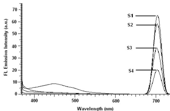
Fig. 7. Fluorescence emission spectra of AuNPs solutions for sample S1-S4.
