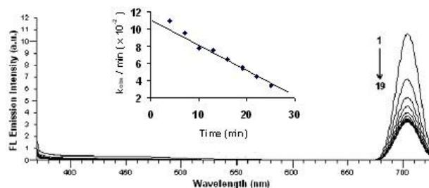
Fig. 8. Fluorescence emission spectra of AuNPs formation with HAuCl<sub>4</sub> (5.16mM)- tea extract(1.5mL) reduction at 3 minutes time intervals. Inset: Plot of  $k_{obs}$  vs. time (min).
