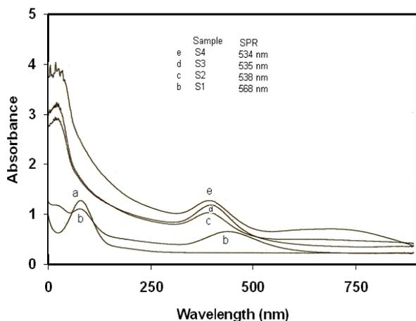
Fig. 5. UV-Visible spectra of (a) aqueous HAuCl<sub>4</sub>, (b-e) AuNPs solutions for sample S1-S 4
