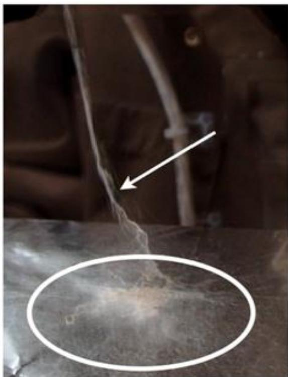
**Fig. 3.** The large floating fibre (indicated by arrow) which is surrounded by smaller floating fibres (indicated by the circle). The fibres are on the collector and the electrospinning needle is above the image.
