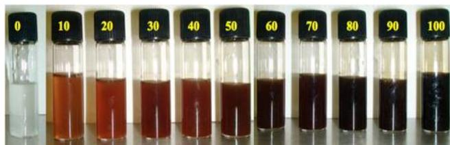
Fig. 1. From left to right, the prepared 0, 10, 20, 30, 40, 50, 60, 70, 80, 90, and 100% lignin solutions.
