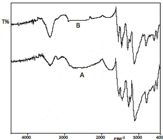
**Fig. 2.** FTIR spectra of PANI/SnO<sub>2</sub> nanocomposites A and B.
