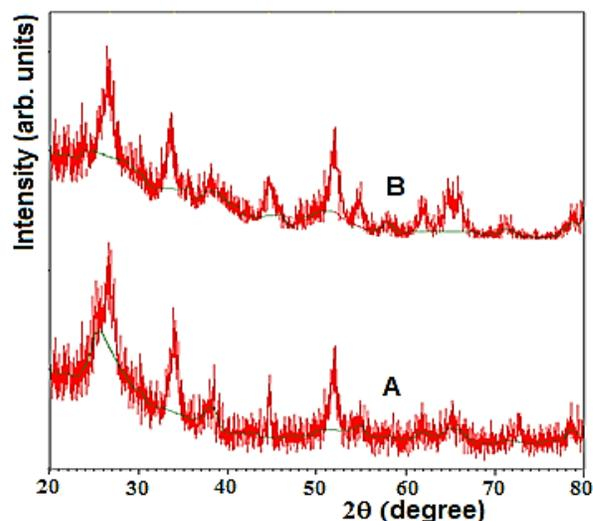
**Fig. 3.** XRD pattern of PANI/SnO<sub>2</sub> nanocomposites A and B.
