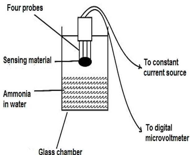
Fig. 4. Four probe laboratory set up for ammonia sensing.
