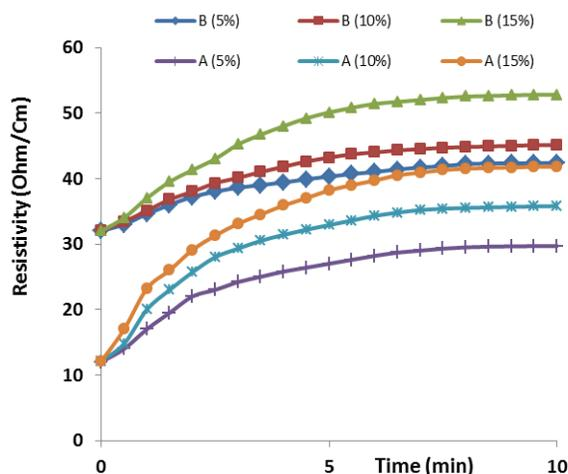
Fig. 5. Resistivity response of PANI/SnO<sub>2</sub> nanocomposites A and B at 5, 10 and 15% concentration of ammonia.
