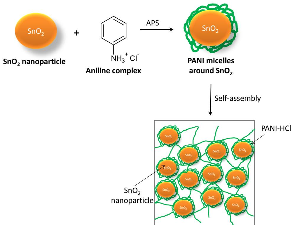
**Scheme 1.** Schematic illustration of PANI/SnO<sub>2</sub> nanocomposite formation.
