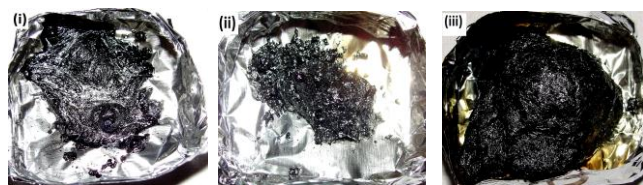
Fig. 6. Digital photographs of residues after heating at 400 °C of (i) PA66, (ii) PA66/NM and (iii) PA66/NM/DMP.
