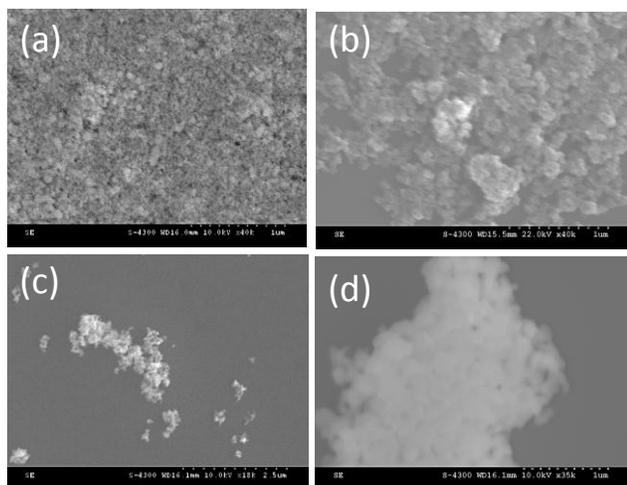
Fig. 3. SEM images of (a) ZrO, (b) Fe<sub>3</sub>O<sub>4</sub>, (c) TiO<sub>2</sub> and (d) Al<sub>2</sub>O<sub>3</sub> particles.
