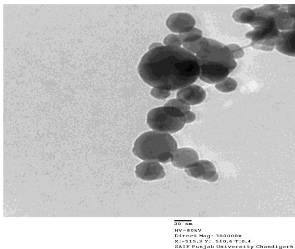
Fig. 4. TEM image of titanium oxide nanoparticles.
