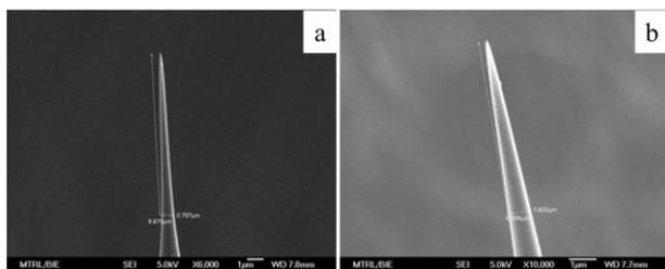
**Fig. 6.** SEM images of nanometer sized tip of optical fiber (a) SEM of condition1 and (b) SEM of condition.
