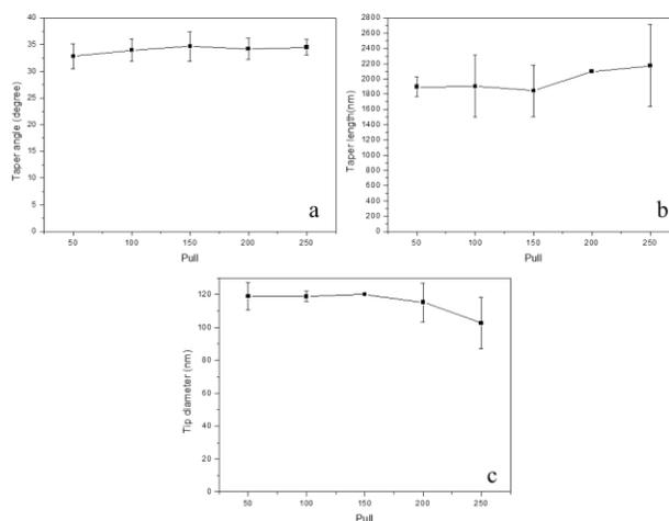
**Fig. 4.** Effect of pull on the optical fiber nanotips (a) pull versus taper angle, (b) velocity versus taper length and (c) pull versus tip diameter.
