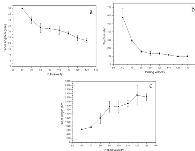
**Fig. 1.** Effect of velocity on the optical fiber nanoprobe (a) velocity versus taper angle, (b) velocity versus tip diameter and (c) velocity versus taper length.
