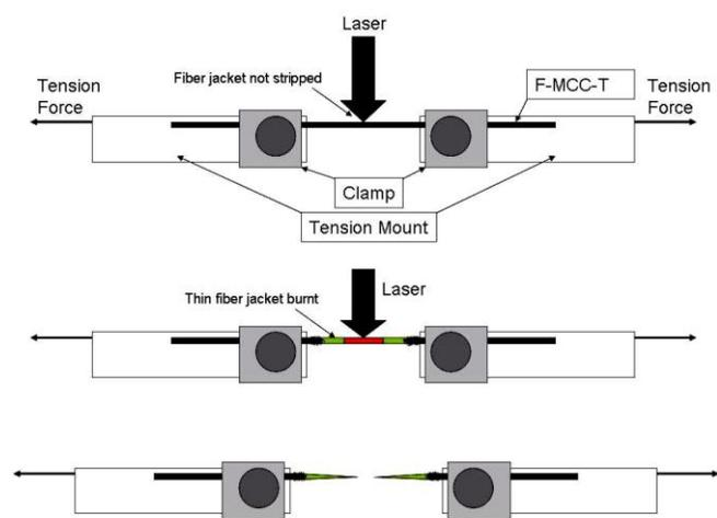
**Scheme 1.** Schematic diagram of the fiber-pulling procedure.
