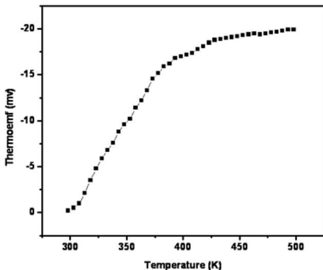
Fig. 6. Plot of Thermoemf Vs Temperature for the MoBi<sub>2</sub>Te<sub>5</sub> thin film.
