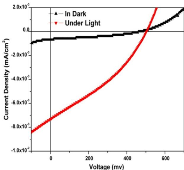
Fig. 7. Plot of voltage (mV) versus current density (mA/cm<sup>2</sup>).
