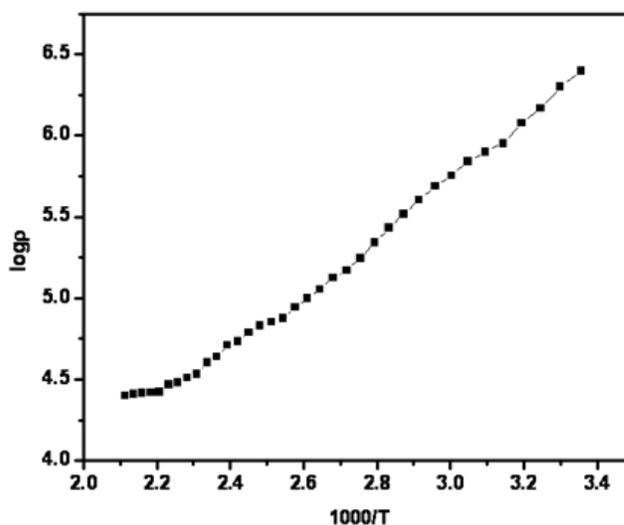
Fig. 5 Plot of  $1000/T$  Vs  $\log \rho$  for  $\text{MoBi}_2\text{Te}_5$  thin film.
