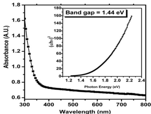
**Fig. 1.** Determination of band gap  $\text{MoBi}_2\text{Te}_5$  thin film.
