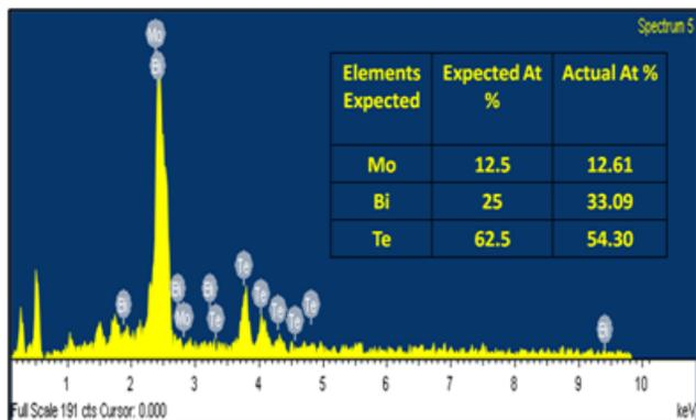
Fig. 3 EDS spectrum of  $\text{MoBi}_2\text{Te}_5$  thin film.
