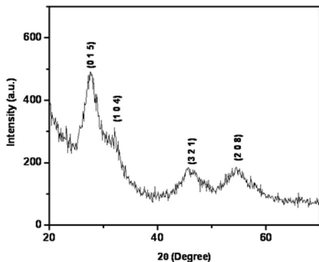
Fig. 4. X-ray diffraction of  $\text{MoBi}_2\text{Te}_5$  thin film.
