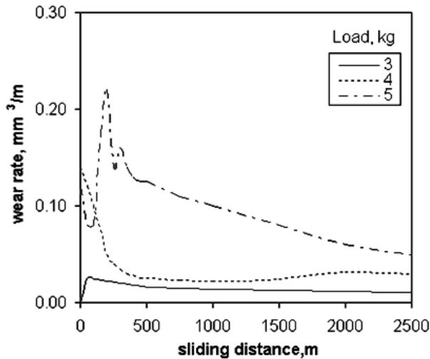
Fig. 2. Variation of wear rate with sliding distance at different loads for alloy 'A' at a temperature of 40 °C.
