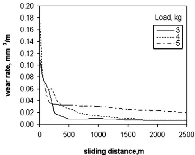
Fig. 3. Variation of wear rate with sliding distance at different loads for alloy 'B' at a temperature of 40 °C.
