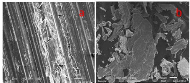
Fig. 9. (a) SEM micrograph of worn surface of as cast alloy 'A' at 80 °C for 4 kg wear load and (b) debris of as cast alloy 'A' at 80 °C for 4 kg wear load.
