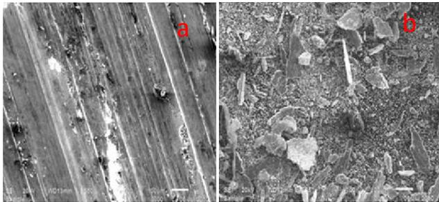
**Fig. 12.** (a) SEM micrograph of worn surface of alloy 'D' at 80 °C for 4 kg wear load. (b) SEM micrograph of debris of alloy 'D' at 80 °C for 4 kg wear load.
