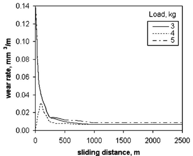
Fig. 5. Variation of wear rate with sliding distance at different loads for alloy 'D' at a temperature of 40 °C.
