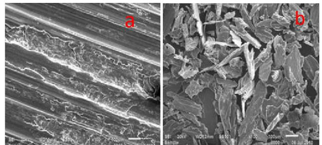
Fig. 10. (a) SEM micrograph of worn surface of alloy 'A' at 80 °C for 4 kg wear load. (b) SEM micrograph of debris of alloy 'A' at 80 °C for 4 kg wear load.
