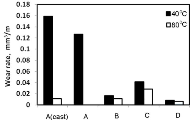
Fig. 8. Wear rate for different alloys at two different temperatures for 5 kg wear load.
