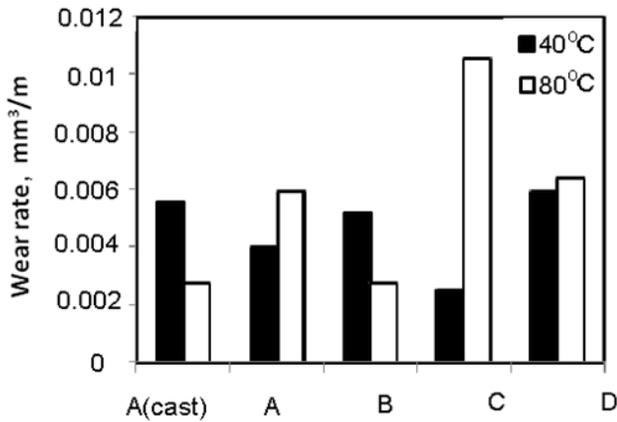
Fig. 6. Wear rate for different alloys at two different temperatures for 3 kg wear load.
