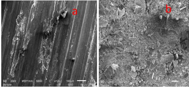
**Fig. 11.** (a) SEM micrograph of worn surface of alloy 'D' at 40 °C for 4 kg wear load. (b): SEM micrograph of debris of alloy 'D' at 40 °C for 4 kg wear load.
