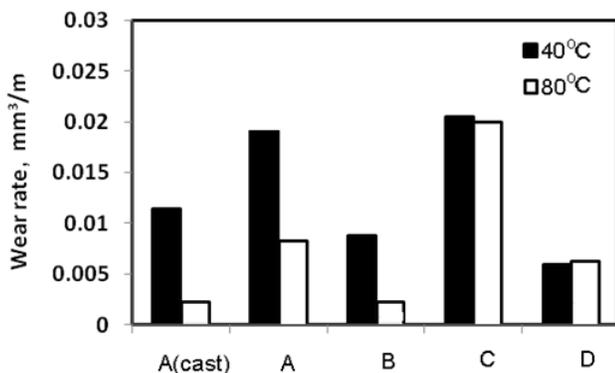
Fig. 7. Wear rate for different alloys at two different temperatures for 4 kg wear load.
