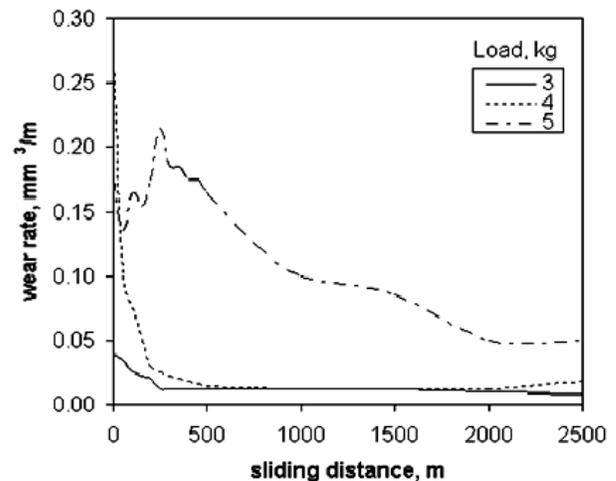
**Fig. 1.** Variation of wear rate with sliding distance at different loads for as cast alloy 'A' at a temperature of 40  $^{\circ}C$ .
