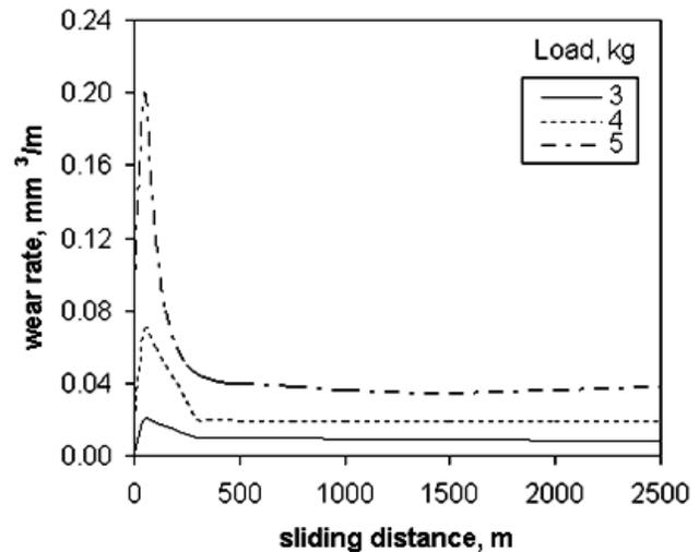
Fig. 4. Variation of wear rate with sliding distance at different loads for alloy 'C' at a temperature of 40 °C.
