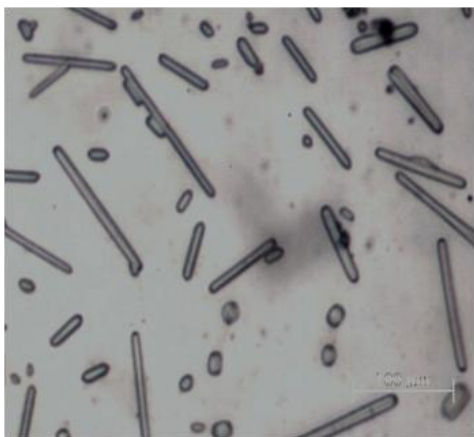
Fig. 5. Microstructure of precipitates of \text{AlB}_2 in aluminium matrix (Expt. 3).
