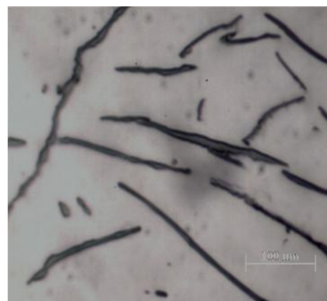
Fig. 1. Microstructure showing flakes of \text{Al}_3\text{Ti} in matrix of aluminium Expt. 2.
