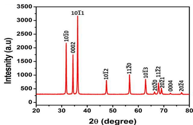
Fig. 1. XRD pattern of the ZnO nanorods.
