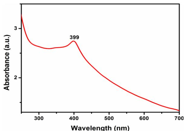
**Fig. 5.** Room-temperature UV-vis absorption spectrum of as-prepared ZnO nanorods.
