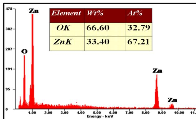
**Fig. 3.** (Color online) EDX spectrum of the synthesized ZnO nanorods by microwave irradiation.
