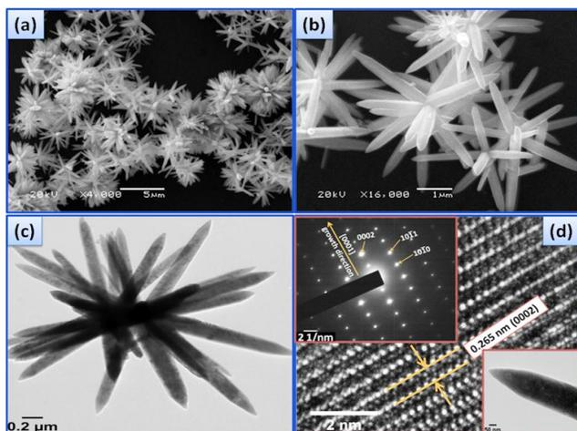
**Fig. 2.** Morphological description of the aggregative ZnO nanostructures: (a) and (b) FESEM images at two different magnifications, TEM micrographs of (c) an individual ZnO nanoflower and (d) HRTEM image of a single nanorod. The upper left and lower right insets in (d) correspond to the SAED pattern and the focused image of a single ZnO nanorod, respectively.
