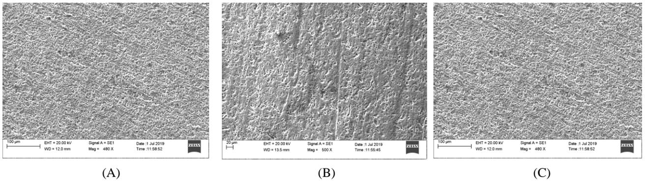
Fig. 5. Base metal Micro structures, (A) Specimen Breaking at high Load, (B) Specimen Breaking at Neck, (C) Specimen Breaking at high Load.
