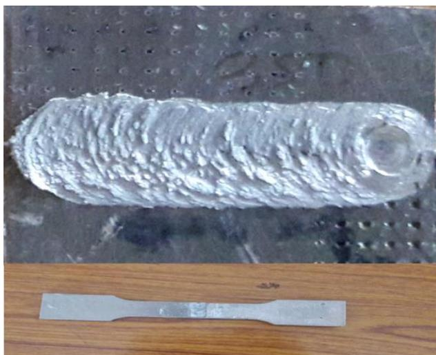
**Fig. 3.** Welded joint & ASTM E8M-04 specimens.
