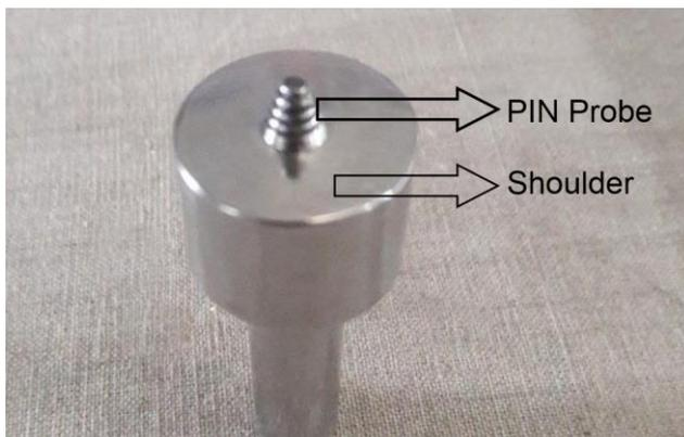
Fig. 1. FSW Tool conical Pin.
