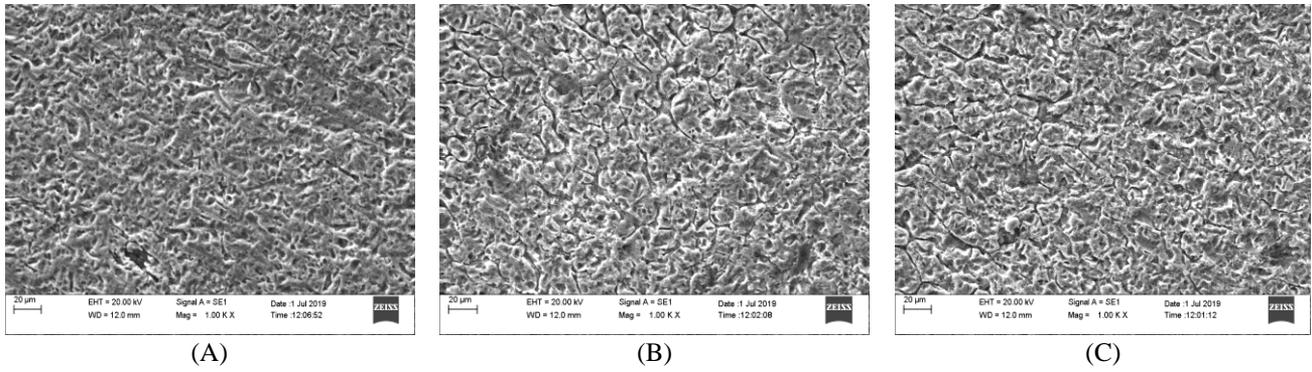
Fig. 4. Welded zone Micro structures, (A) Specimen Breaking at high Load, (B) Specimen Breaking at Neck, (C) Specimen Breaking at high Load.
