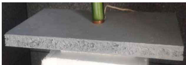
Fig. 7. A tested sample of aluminium foam with dimensions 290 × 130 × 15 mm and apparent density 0.547 g/cm 3 .
