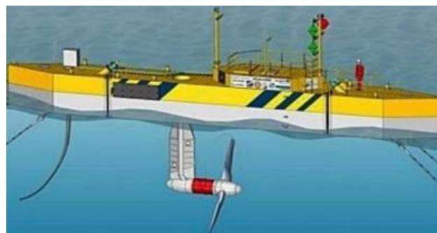
Fig. 9. Recent Tidal turbine configuration to simplify repairing [20].
