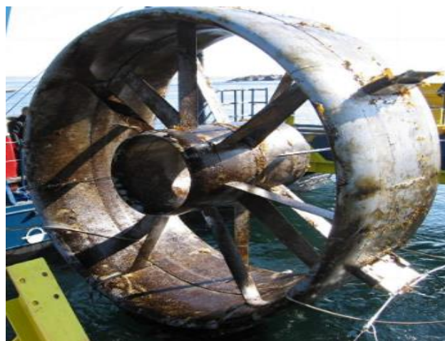
Fig. 5. Some Biofouling accumulated on tidal turbines [21].
