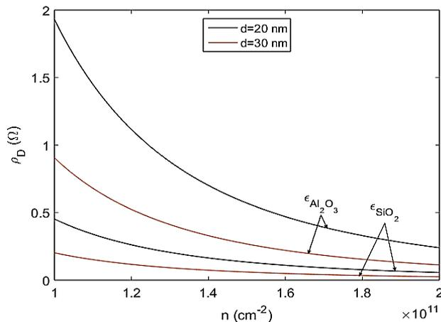
Fig. 3. The schematic diagram show the dependence of the resistivity  $\rho_D$  with the concentration for the GaAs quantum well at temperature  $T=10$  k.
