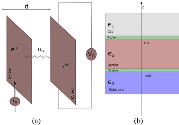
**Fig. 1.** Schematic drawing of the experimental geometry. The current  $I_A$  is applied from the active layer, and the voltage difference  $V_D$  is induced in passive layer as shown in Fig. (1a). Schematic geometry illustration considered in Fig. (1b). The 2DEG is located within a QW and is defined by active and passive for its position along the  $z$  direction. The structure's relative dielectric constants are given by  $\epsilon_1, \epsilon_2, \epsilon_3$  as shown in Fig. (1b).
