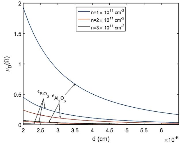
Fig. 4. Schematic diagram show the behaviour of the  $\rho_D$  with interlayer separation  $d$  for the system of *air/GaAs/SiO<sub>2</sub>/GaAs/AlGaAs* as shown.
