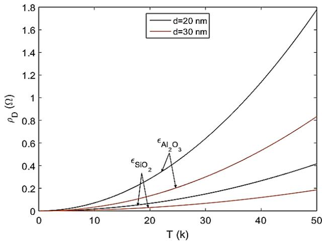
Fig. 2. The schematic diagram show the dependence of the resistivity  $\rho_D$  with the temperature  $T$  (at low temperature ( $T \ll T_F$ ) as shown in figure for the GaAs quantum well with carrier concentration  $n = 2 \times 10^{11} \text{ cm}^{-2}$ . The curves also show the dependence of the dielectric constant of the barrier ( $\text{SiO}_2$  ( $\epsilon_2 = 4$ ) and  $\text{Al}_2\text{O}_3$  ( $\epsilon_2 = 4$ )) and interlayer distance ( $d=20$  nm and  $30$  nm).
