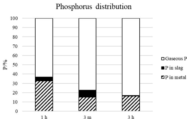
**Fig. 6.** Phosphorus degree obtained in inductively heated graphite bed reactor [19].
