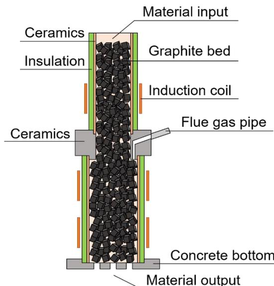
Fig. 2. Inductively heated bed of graphite pieces [22].
