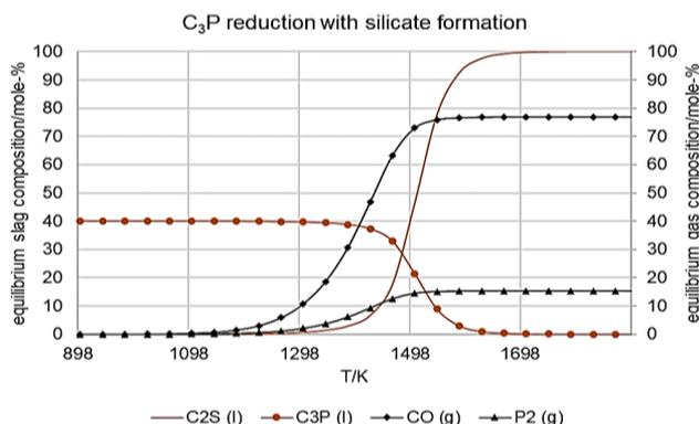
Fig. 1. Direct reduction of C<sub>3</sub>P considering the involvement of SiO<sub>2</sub> [19].
