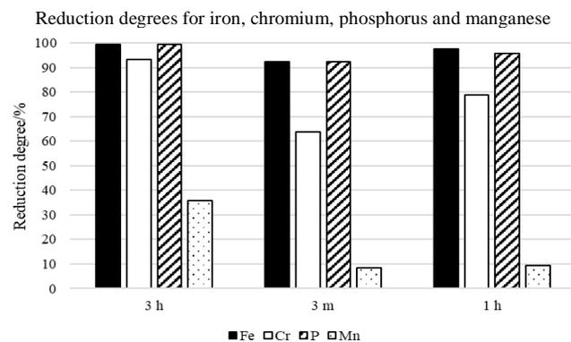
**Fig. 5.** Reduction degrees obtained by treatment in the inductively heated graphite bed reactor [19].
