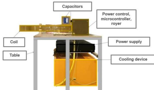
Fig. 10. Induction furnace used for smelting and reduction experiments.
