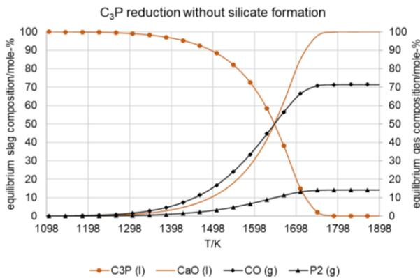
Fig. 8. Direct reduction of C<sub>3</sub>P not considering the involvement of SiO<sub>2</sub> [19].
