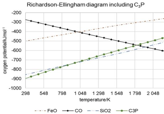
Fig. 7. Position of C<sub>3</sub>P in a Richardson-Ellingham diagram [19].
