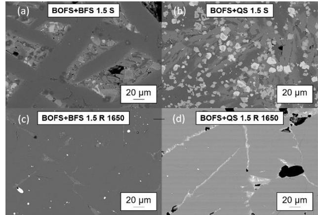
Fig. 11. SEM images of produced slag samples: (a) BOFS+BFS, B<sub>2</sub>=1.5, smelting step (b) BOFS+QS, B<sub>2</sub>=1.5, smelting step (c) BOFS+BFS, B<sub>2</sub>= 1.5, reduction at 1,923 K (d) BOFS+QS, B<sub>2</sub>=1.5, reduction at 1,923 K.
