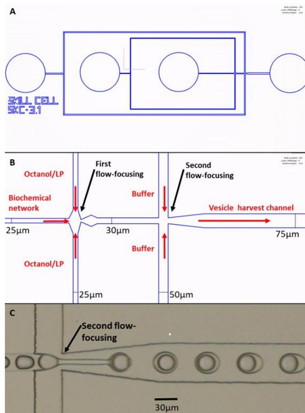
Fig. 4. Microfluidic method for Giant Unilamellar Vesicle (GUV) production containing biochemical networks. (A) Overview of SKC3.1 design. (B) GUV are produced by two consecutive flow focusing pointed by black arrows. Width dimensions of channels are shown and flow directions are indicated by red arrows. (C) Flow focusing showing the formation of double emulsion vesicles. W/O/W vesicles are formed with an excess of 2-octanol that are released spontaneously in a post-production step.
