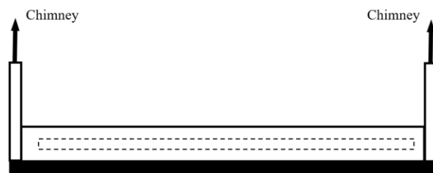
Fig. 3. Schematic description of a twin rail carburizing box using coal as a carburizing agent and oxy-acetylene flame to avoid decarbonizing. Source: own
