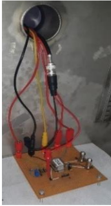
Fig. 6. The image showing the wires which contain the data come out of the hole which is placed left side of the oven and these wires are connected to the computers and power supplies.
