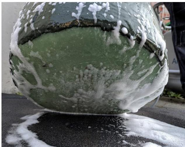
**Fig. 1.** Leakage throughout the GFRP structure of a small-scale tank prototype at 1 bar (relative) after undergoing several thermal cycles from room temperature to 77 K and back.
