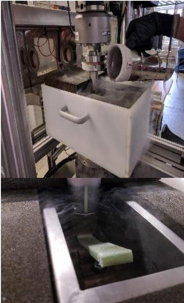
Fig. 4. Three-point-bending test stand for cryogenic testing.
