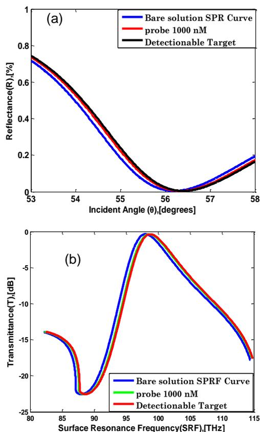
**Fig. 2.** Numerical results of Bare SPR Sensor (a)  $R_{\sim}SPR\text{-angle}$  curve in the absence of formalin and chitosan. (b)  $T_{\sim}SPRF$  curve in the absence of formalin and chitosan.
