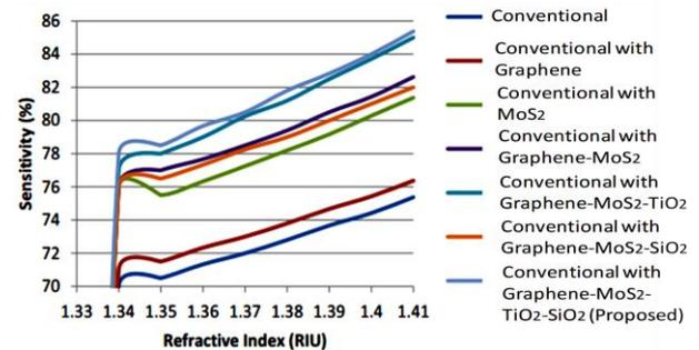
**Fig. 4.** Sensitivity [%] vs. Refractive Index [RIU] graph for different Layer Structure.
