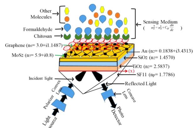
Fig. 1. Schematic of Graphene-MoS<sub>2</sub>-Au-TiO<sub>2</sub>-SiO<sub>2</sub> Model for Mechanism of Formalin Detection with Hybrid Layer Biosensor.
