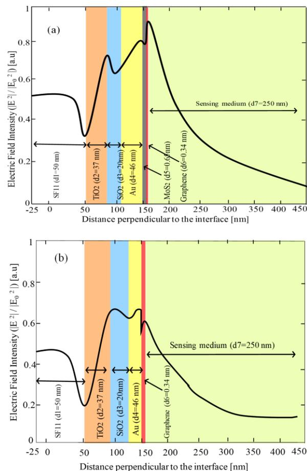
**Fig. 5.** The electric field intensity in the direction of x axis along the perpendicular to the interface for the structure (a) with MoS<sub>2</sub> layer and (b) without MoS<sub>2</sub> layer.
