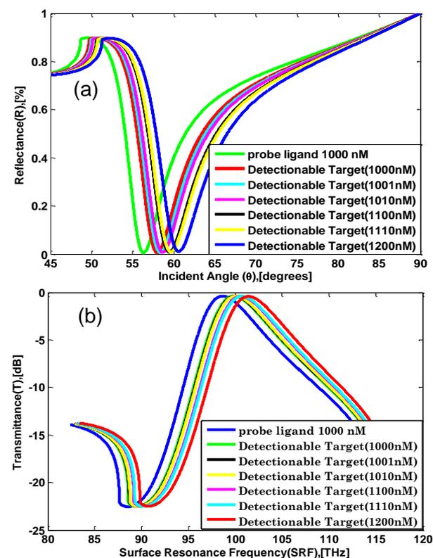
**Fig. 3.** (a) Reflectance vs. Incident Angle Curve and (b) Transmittance vs. SPR Frequency Curve for Different Concentration of Detectionable Target.
