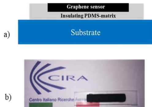
Fig. 1. Schematic (a) and picture (b) of the PDMS-G strain sensor.
