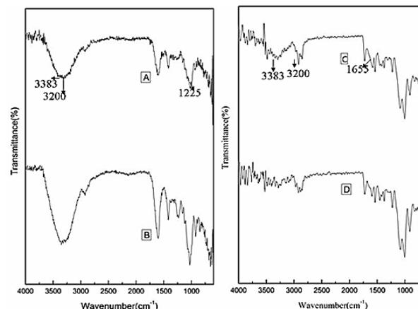
Fig. 1. FTIR spectra of (A) alginate/ $\kappa$ -Car, (B) curcumin loaded alginate/ $\kappa$ -Car, (C) alginate/gelatin, (D) curcumin loaded alginate/gelatin hydrogel beads.
