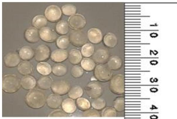
Fig. 2. Morphological analysis of hydrogel beads.
