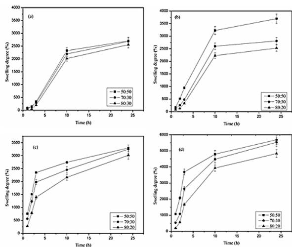
**Fig. 4.** Effect of alginate/gelatin weight ratio's on the swelling of the alginate/gelatin composite. Hydrogel beads at different polymer concentrations (a) 1.5% (b) 2.5% and effect of alginate/ $\kappa$ -Car weight ratio's on the swelling of the alginate/ $\kappa$ -Car hydrogel beads with polymer concentrations (a) 1.5% (b) 2.5%.
