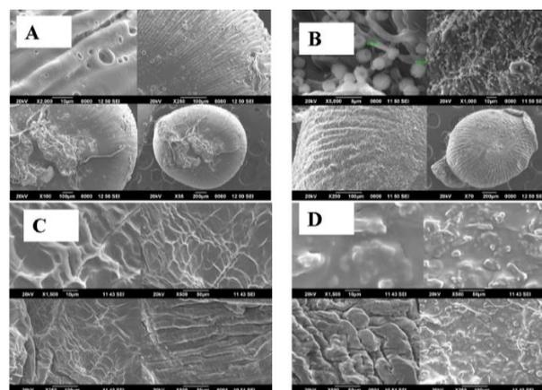
Fig. 3. SEM micrographs of unloaded (a) alginate/ $\kappa$ -Car, (b) alginate/gelatin hydrogel beads and curcumin loaded (c) alginate/ $\kappa$ -Car (d) alginate/gelatin hydrogel beads.
