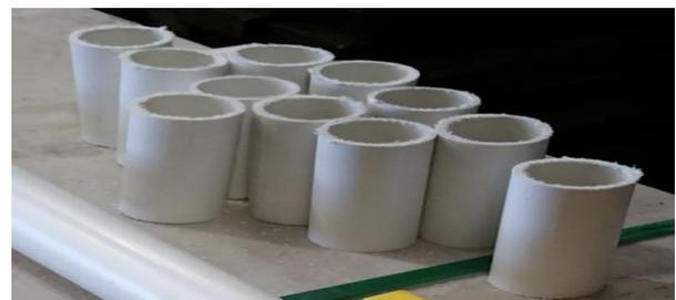
**Fig. 2.** PVC moulds.
