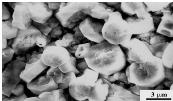
Fig. 4. SEM photograph of the specimen with \text{Na}_{3.9}\text{Sm}_{0.6}\text{P}_{0.3}\text{Si}_{2.7}\text{O}_9 composition heated at 900 °C by the pattern (c).
