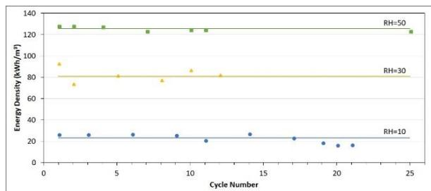
**Fig. 4.** Experimental energy density of multi-cycle breakthrough experiments using 80 °C regeneration temperature for different inlet RH.
