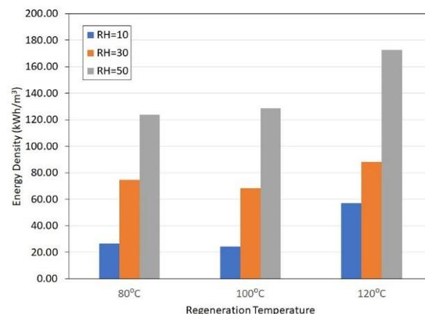
**Fig. 3.** Experimental energy density of silica gel sample measured at different inlet RHs and regeneration temperatures.
