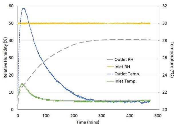
**Fig. 2.** Relative humidity and temperature breakthrough curves for silica gel packed column using 100°C regeneration temperature and 50% inlet RH.
