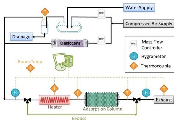
Fig. 1. Schematic illustration of the adsorption thermal energy storage system.
