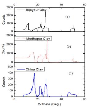
Fig. 4. XRD analysis of Bijoypur Clay (a) [1], Modhupur Clay (b) [1] and China Clay (c) [7].
