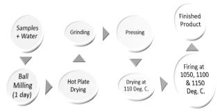
Fig. 3. Flow diagram of tile samples preparation from locally available raw materials.
