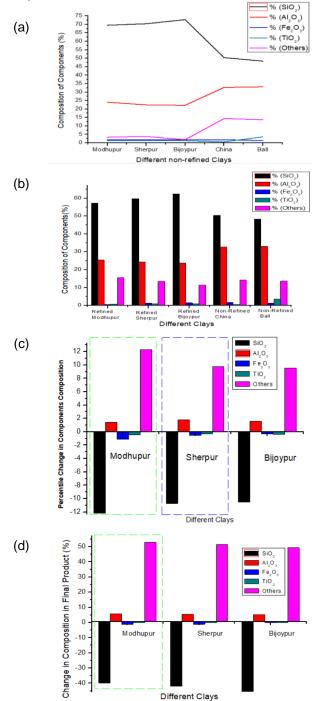
**Fig. 5.** (a) Non-refined Samples composition, (b) Refined local clay samples in contrast to imported china and ball clay, (c) Percentile point change in new refined local clay samples and (d) Change in composition in refined local clay samples from the non-refined samples.
