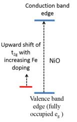
Fig. 8. Formation of Energy band gap of Fe doped in NiO NPs.
