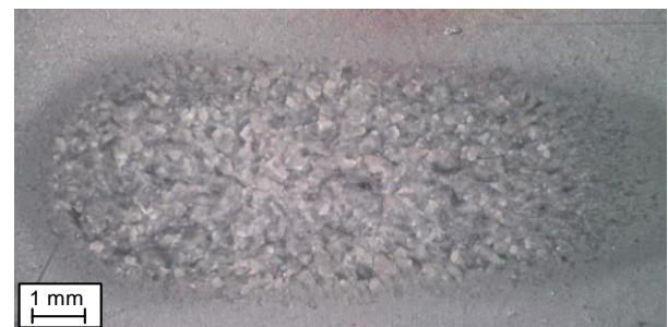
Fig. 7. Cutting surface at AlMg3 for liquid CO 2 with CO 2 -microcrystals as abrasive.
