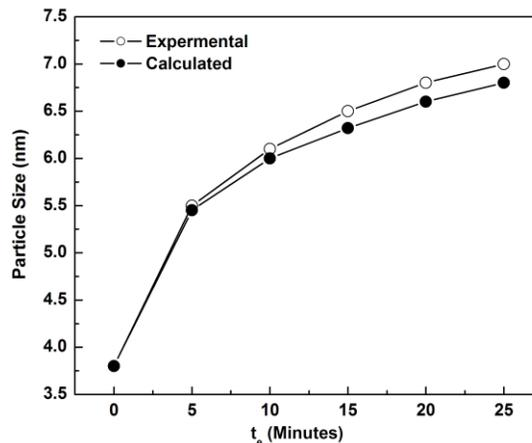
Fig. 5. Variation of theoretically calculated and experimentally observed growth of Au nanoparticles with electron irradiation time.
