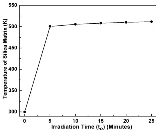
Fig. 4. Calculated curve for rise in temperature of silica matrix due to electron beam heating effect at current density  $1.78 \times 10^8 \text{ A/m}^2$ .
