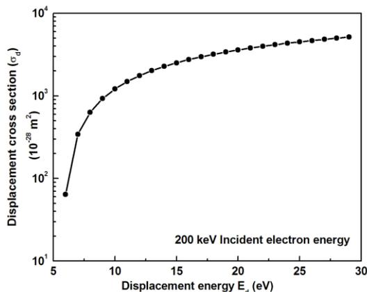
Fig. 3. Variation of displacement cross-section for different displacement energies for 200keV electron beam irradiation.
