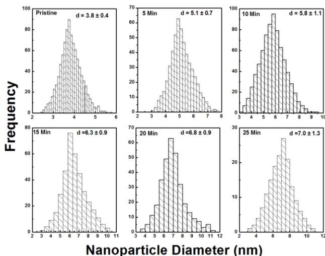
**Fig. 2.** Size distribution (a-f) of Au nanoparticles for (a) pristine and (b-f) irradiated for different times. Frequency is in arbitrary unit.
