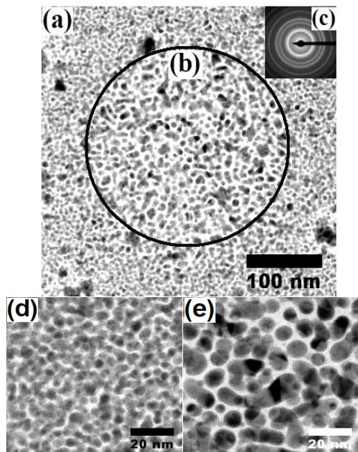
**Fig. 1.** Bright field TEM image of (a) pristine sample and (b) section of (a) irradiated with electron beam. Picture (c) shows the electron diffraction pattern. (d) and (e) are the magnified view of TEM images of pristine and electron irradiated sample up to 25 minutes, respectively.
