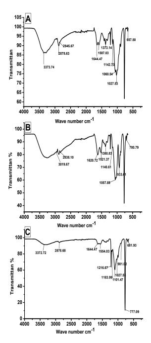
**Fig. 1.** IR spectra of (A) Chitosan (B) Ch-g-sty (C) styrene grafted chitosan loaded by chromium.
