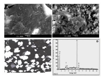
**Fig. 4.** SEM-EDX analysis of (A) Chitosan (B) Ch-g-sty (C) ch-g-sty loaded by chromium (D) EDX graph of styrene grafted chitosan loaded by chromium.
