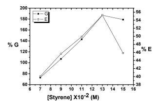
Fig. 7. % G and % E with changing monomer concentration at fixed concentration of chitosan (0.1 g/25 mL), 80 % MW power, 40 sec exposure time.
