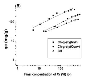
Fig. 11. Adsorption equilibrium (A) langmuir and (B)Frundlich Isotherm on various adsorbents Plain Chitosan (CH), conventional synthesized (Ch-g-sty) and Microwave synthesized (Ch-g-sty). (T = 303 K, pH = 3).
