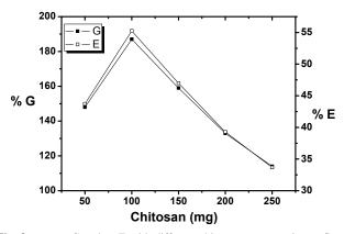
**Fig. 8.** % G and % E with different chitosan concentration at fixed concentration of styrene (13 x  $10^{-2}$  M) 80 % MW power and 40 sec exposure time.
