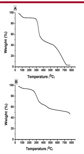
Fig. 3. TGA analysis of (A) Chitosan (B) Ch-g-sty.
