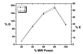
**Fig. 6.** %G and %E with exposure time at the fixed concentration of styrene (13 x  $10^{-2}$ ), chitosan (0.1 g/25 mL) at 80 % MW power.
