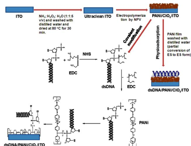
Fig. 2. Schematic presentation of proposed electrochemical DNA biosensor.
