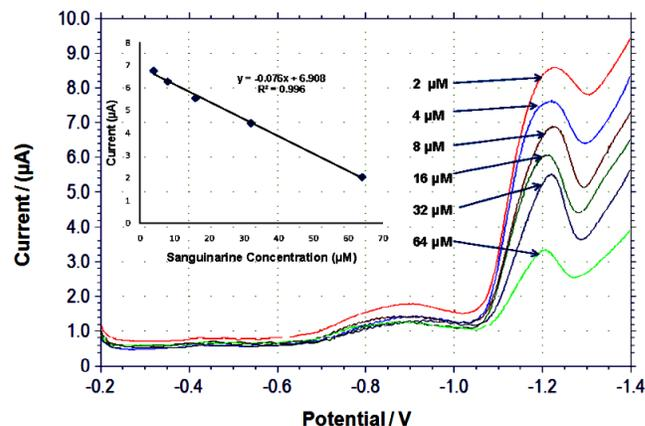
**Fig. 7.** DPV Shows the effect of sanguinarine at various concentrations using covalently modified dsDNA onto PANi/ClO<sub>4</sub> film format in 0.1 M PBS pH 7.0. Inset shows calibration plot of sanguinarine vs. current.
