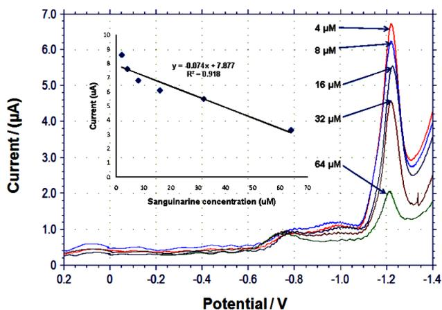
**Fig. 6.** DPV Shows the effect of sanguinarine at various concentrations using physioadsorbed dsDNA onto PANi/CIO<sub>4</sub> film in 0.1 M PBS buffer pH 7.0. Inset shows calibration plot of sanguinarine vs. current.
