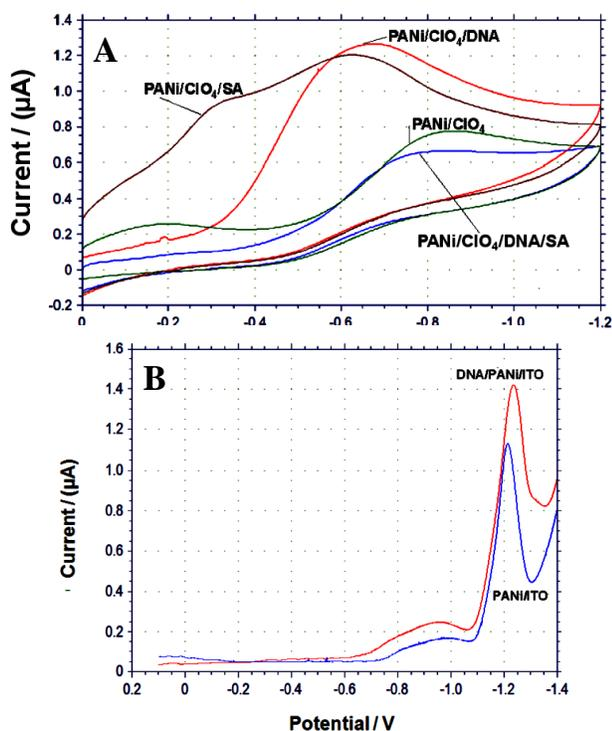
**Fig. 1.** (A) Cyclic Voltammograms show interaction study of sanguinarine with and without dsDNA using sanguinarine (16 µM) alone and sanguinarine (16 µM) with covalently modified DNA onto the film of PANi in 0.1 M PBS buffer, pH 7.0 and (B) Differential Pulse Voltammetry shows the PANi/ITO film and DNA/PANi/ITO film trend in 0.1M PBS solution, pH 7.0.
