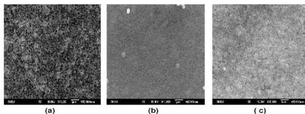
**Fig. 5.** Shows SEM image (a) ITO/ PANi/CIO<sub>4</sub> film (b) ITO/PANI/CIO<sub>4</sub>/dsDNA film; physically adsorbed and (c) ITO/PANI/CIO<sub>4</sub>/dsDNA film; Covalently (EDC/NHS) modified.
