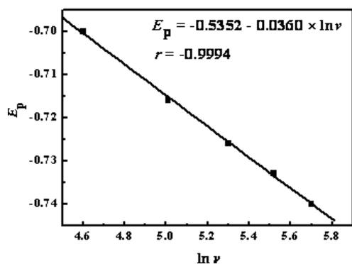
**Fig. 7.** The relationship between  $E_p$  and  $\ln v$ .
