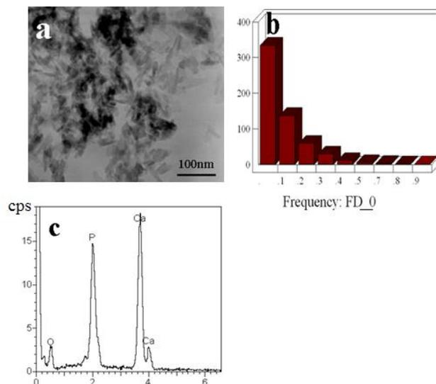
**Fig. 1.** (a) TEM image of HAp, (b) The distributing size of granule separated by ultrasonic, (c). Compositional information of HAp obtained through EDS analysis.
