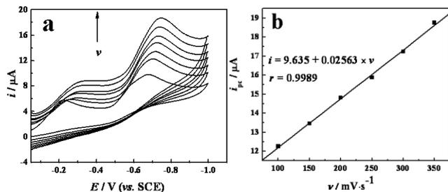
**Fig. 6.** (a) CV curves of dsDNA/HAp/GCE in  $5.0 \times 10^{-5} \text{mol}\cdot\text{L}^{-1}$   $\text{VB}_{12}$  solution with different scan rates of 50, 100, 150, 200, 250, 300 and 350  $\text{mV}\cdot\text{s}^{-1}$  respectively, (b). The dependence of the peak currents on scan rates.
