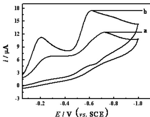
**Fig. 3.** CV curves of dsDNA/HAp/GCE (curve a) and GCE (curve b) in  $5 \times 10^{-5} \text{ mol}\cdot\text{L}^{-1} \text{ VB}_{12}$  solution; scan rate,  $100 \text{ mV}\cdot\text{s}^{-1}$
