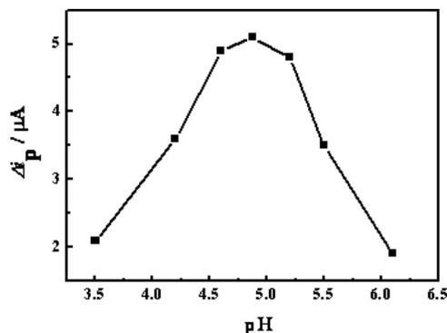
**Fig. 5.** The relationship between  $\Delta i$  and pH
