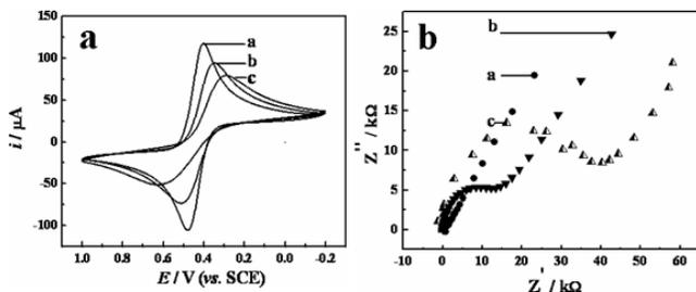
**Fig. 2.** CV (a) and EIS (b) of GCE (curve a), HAp/GCE (curve b) and dsDNA/HAp/GCE (curve c) in  $6.67 \text{ mmol}\cdot\text{L}^{-1} \text{ K}_3[\text{Fe}(\text{CN})_6]$  solution containing  $\text{KNO}_3$  supporting electrolyte; scan rate,  $100 \text{ mV}\cdot\text{s}^{-1}$ .
