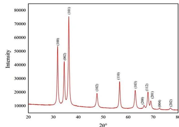
Fig. 1. PXRD pattern of ZnO NPs.
