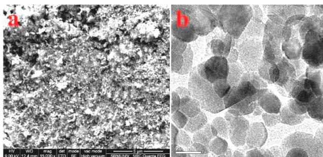
Fig. 3. (a) FE-SEM and (b) HRTEM images of ZnO NPs.
