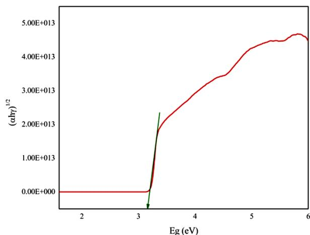
Fig. 2. Evaluation of band gap energy of ZnO NPs.
