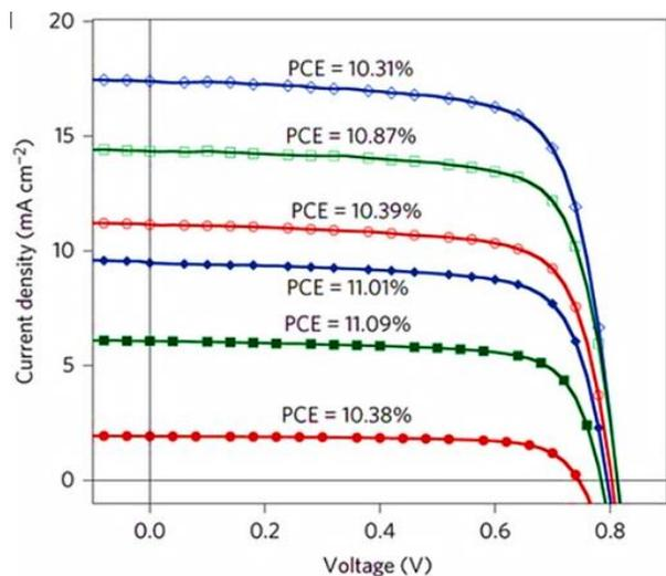
**Fig. 2.** J–V characteristics of a device with 65 wt % PC<sub>71</sub>BM in the active layer tested under different illumination conditions (as obtained from standard AM 1.5G, 1,000 W m<sup>-2</sup> illumination using a set of neutral optical filters) [29] (Nature Photonics, Copyright © 2015, Nature Publishing Group).
