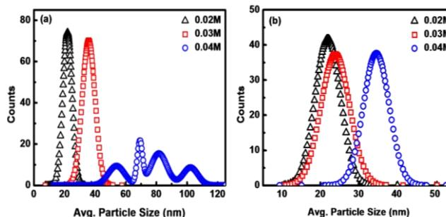
Fig. 2. Average particle size Gaussian distribution of (a) as deposited and (b) annealed sample for different molar concentrations of the solutes.
