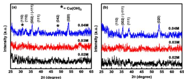
**Fig. 3.** XRD pattern for (a) as deposited and (b) annealed sample of 0.02M, 0.03M and 0.04M.
