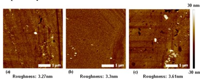
**Fig. 4.** Surface morphology of CuO nanoparticle thin film for (a) 0.04M, (b) 0.03M and (c) 0.02M bath solution.
