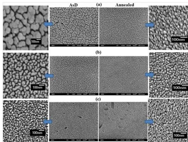
Fig. 1. SEM image of CuO the nanoparticle thin film for as-deposited (Left side) annealed sample (right side) for (a) 0.04M, (b) 0.03M and (c) 0.02M bath solution.
