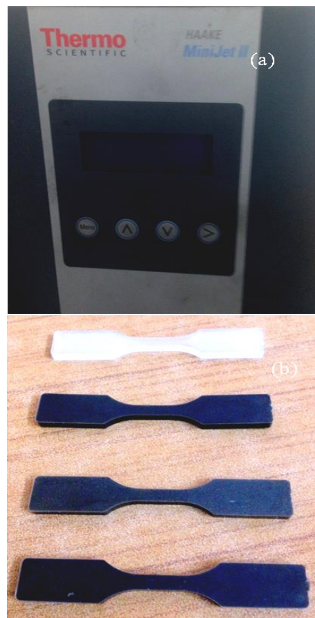
Fig. 2. (a) Injection Molding Machine (Thermo scientific Haake MiniJet) (b) Dumbbell shaped samples for tensile testing.
