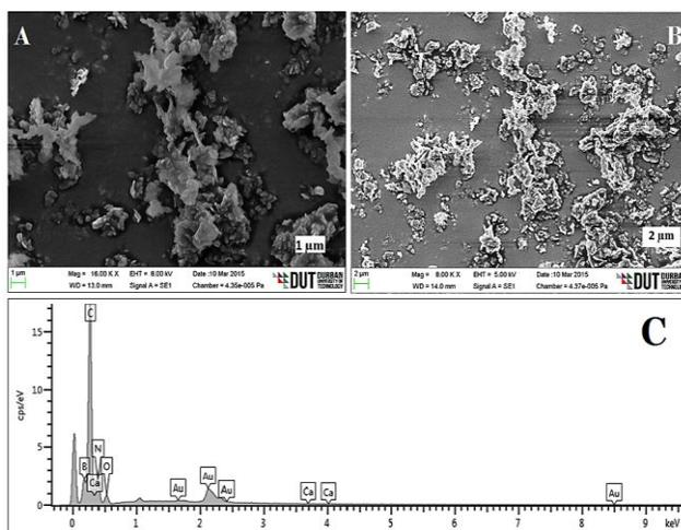
**Fig. 2.** SEM image for calcium loaded boron nitride at  $1\ \mu\text{m}$  (A) and  $2\ \mu\text{m}$  (B) and EDX spectrum (C).
