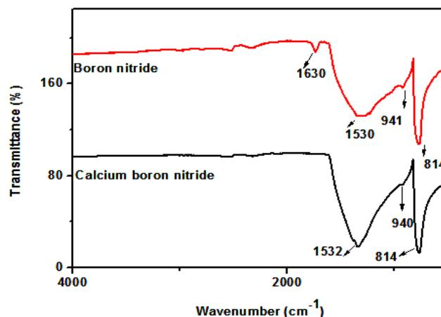
Fig. 6. FT-IR spectrum for calcium loaded boron nitride catalyst.
