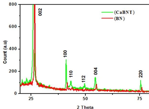
**Fig. 1.** XRD characterization for calcium loaded boron nitride catalyst.
