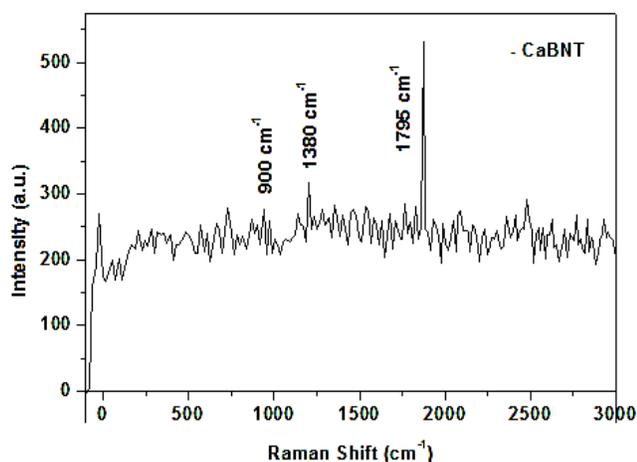
Fig. 4. Raman spectrum for calcium loaded boron nitride.
