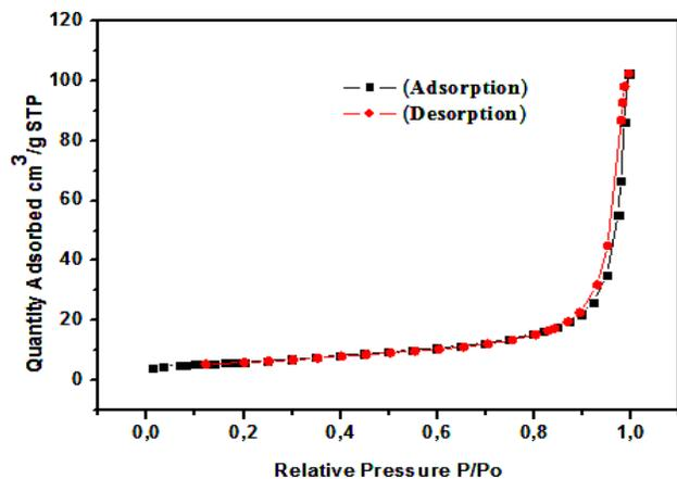
Fig. 3. BET surface area and surface size for calcium loaded boron nitride.
