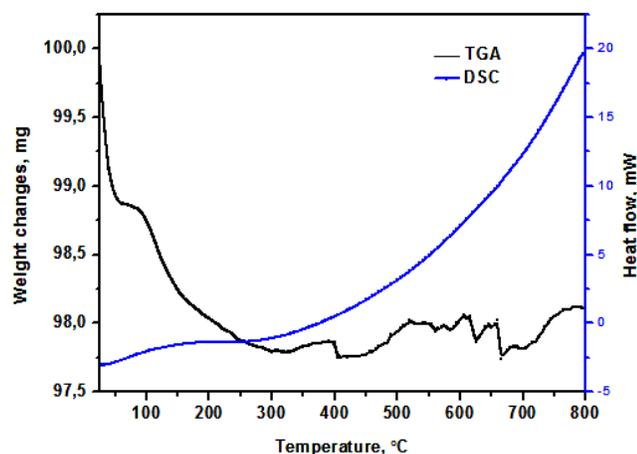
Fig. 5. DSC-TGA for calcium loaded boron nitride catalyst.
