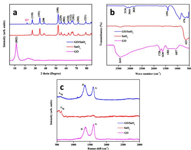
**Fig. 2.** (a) XRD pattern of GO, SnO<sub>2</sub> and SnO<sub>2</sub>/GN, (b) FT-IR spectra of GO, SnO<sub>2</sub> and SnO<sub>2</sub>/GN and (c) Raman spectra of GO, SnO<sub>2</sub> and SnO<sub>2</sub>/GN nanocomposite.
