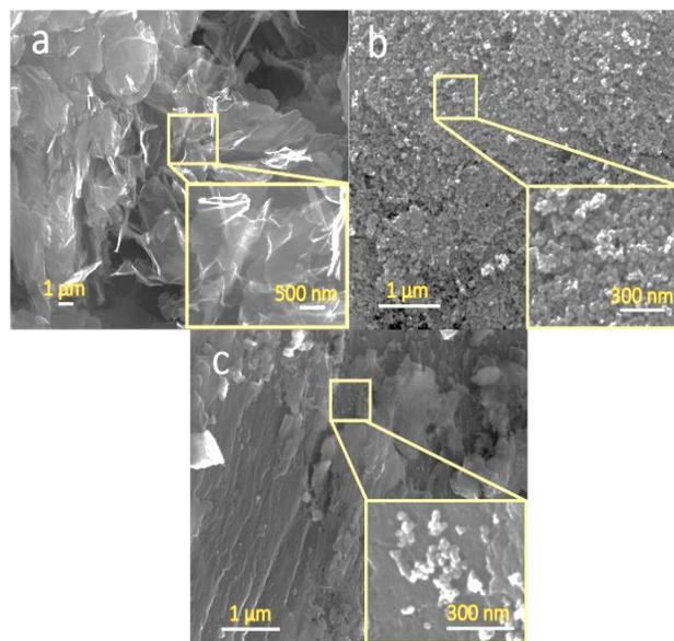
**Fig. 1.** FE-SEM image of (a) GO, (b) SnO<sub>2</sub> and (c) SnO<sub>2</sub>/GN nanocomposite.
