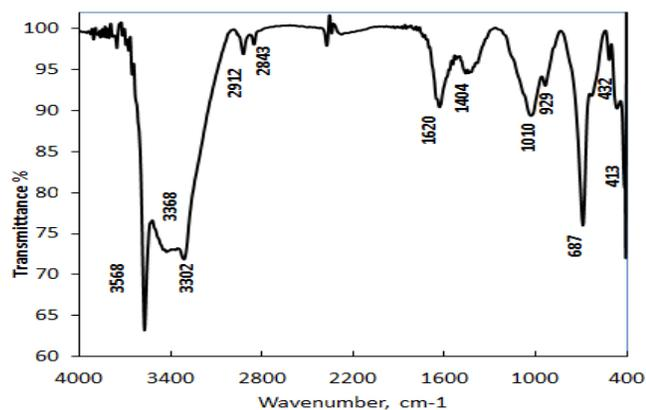
**Fig. 2.** FT-IR spectra of synthesized copper hydroxide nanowires.
