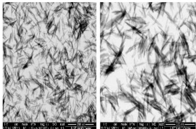
**Fig. 5.** SEM bright field image of the synthesized copper hydroxide nanowires.
