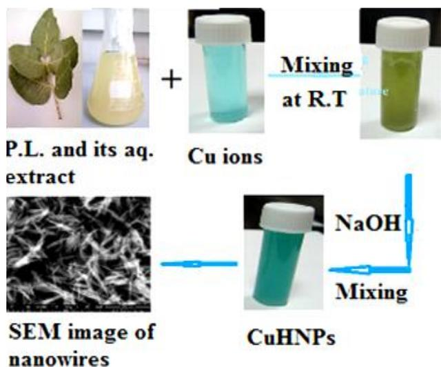
**Scheme 1.** Schematic representation for synthesis copper hydroxide nanowires.
