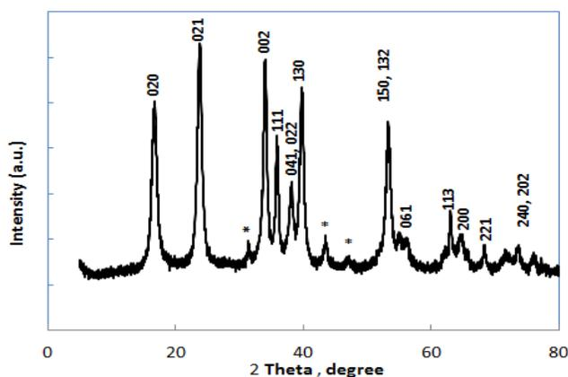
**Fig. 1.** XRD pattern of the synthesized copper hydroxide nanowires.
