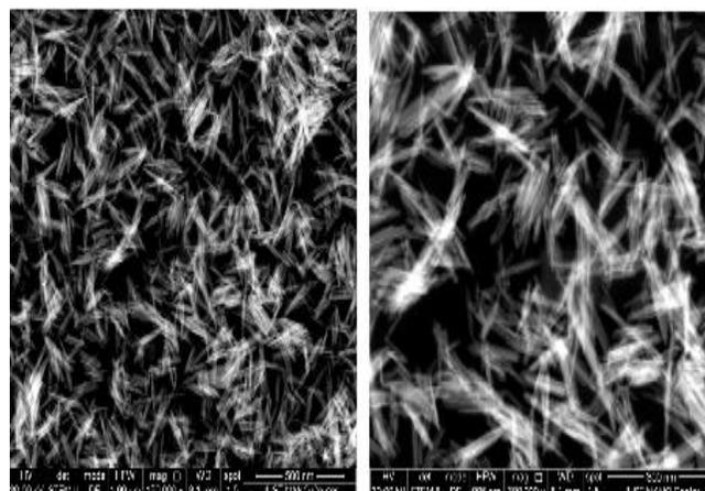
**Fig. 4.** SEM dark field image of the synthesized copper hydroxide nanowires.
