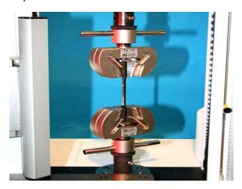
Fig. 4. Tensile test machine Instron 5566-CN2081.
