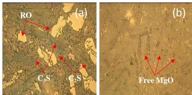
**Fig. 1.** Lithofacies photograph of original steel slag of (a) 1% NH<sub>4</sub>Cl solution erosion ( $\times 400$ ), and (b) uncorroded ( $\times 400$ ).
