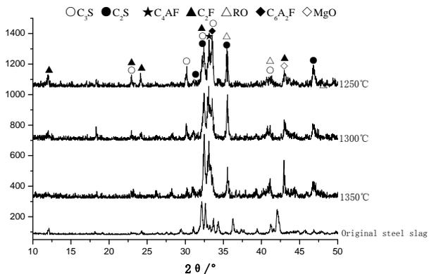
Fig. 3. X-ray diffraction patterns of steel slag which by different temperature treatment.
