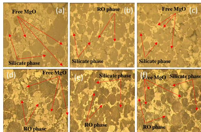
**Fig. 2.** Lithofacies photograph of steel slag at (a) 1250°C uncorroded ( $\times 400$ ), (b) 1300°C uncorroded ( $\times 400$ ), (c) 1350°C uncorroded ( $\times 400$ ), (d) 1250°C 1% NH<sub>4</sub>Cl solution eroded ( $\times 400$ ) (e) 1300°C 1% NH<sub>4</sub>Cl solution eroded ( $\times 400$ ) and (f) 1350°C 1% NH<sub>4</sub>Cl solution eroded ( $\times 400$ ).
