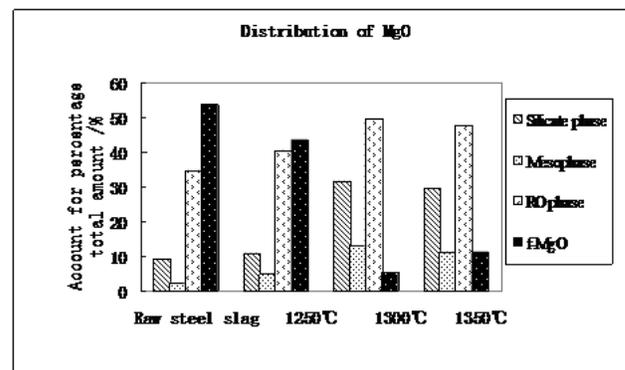
Fig. 5. Distribution of MgO in reconstructird steel slag which by different temperature treatment.
