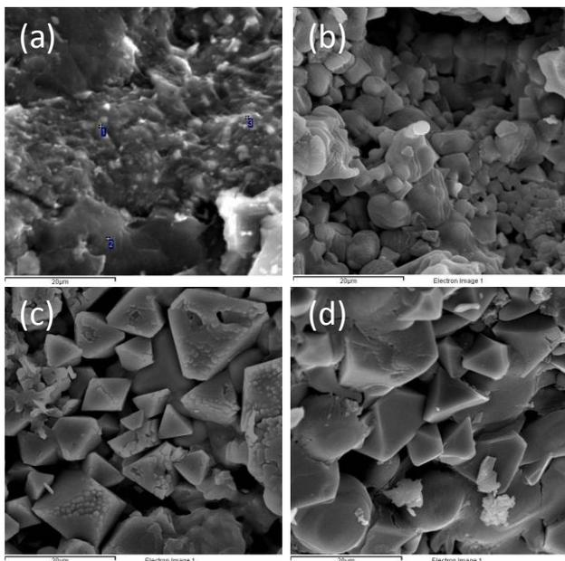
Fig. 4. SEM photograph of steel slag which by different reconstruction temperature treatment.
