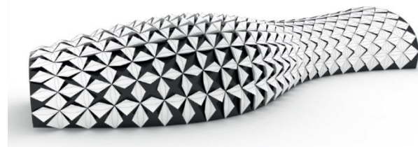
Fig. 1. Scheme of a doubly curved window façade completely covered by Flectofold elements (detailed view of Flectofold element in Fig. 3).
